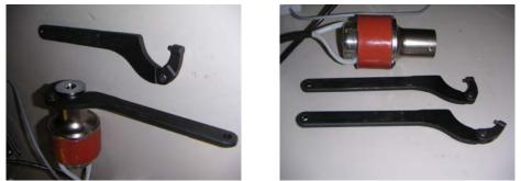
For fixation (screwing, unscrewing) of converter and wave-guide use here presented wrenches.
