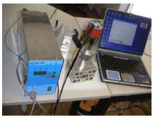
Picture of the complete ultrasonic system configuration: MMM-Generator (left), Converter-Wave-guide-Water-jacket-Aluminum block (middle) and PC (right). PC Interface RS485 to RS232 is connected between the PC and MMM generator. Client should use his own PC. Software **msg\_ix.exe** for the MSG.1200.IX should be installed (download software here:
